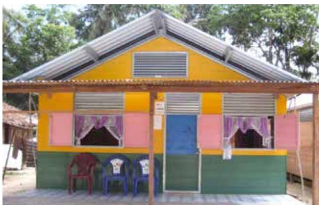
← Permanent houses provided by the Canadian Red Cross in Aceh, Indonesia, were 44m<sup>2</sup>, each consisting of four rooms and a kitchen. The houses were designed for construction in accordance with the requirements of earthquake zone 6 in the Indonesian design code. All housing was constructed to be 30cm above the high water mark.
